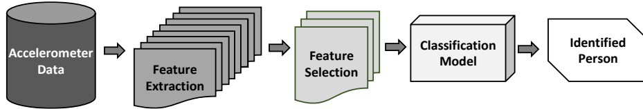
Figure 1. ML approach for person identification using the acceleration signal produced by a door movement.
